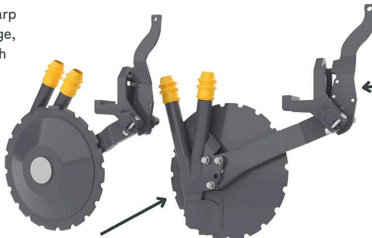
The couler's sturdy attachment to the frame and strong steel plate arms make the structure durable and long-lasting.
