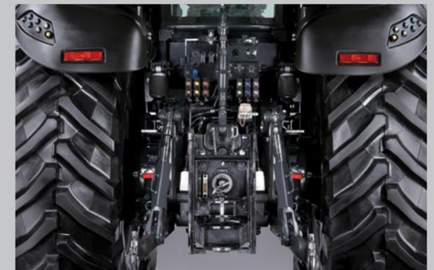
12,000 kg lifting capacity, 210 l/min pump output, three PTO speeds: designed to master any implement.
